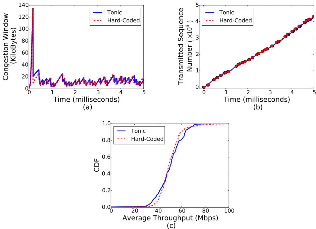
Figure 2.3: NewReno’s Tonic vs hard-coded implementation in NS3 (10G line-rate): a) Congestion window updates (single flow, random drops), b) Transmitted sequence numbers with retransmission in large dots (single flow, random drops), and c) CDF of average throughput of multiple flows sharing a bottleneck link over 5 seconds (200 flows from 2 hosts to one receiver)
