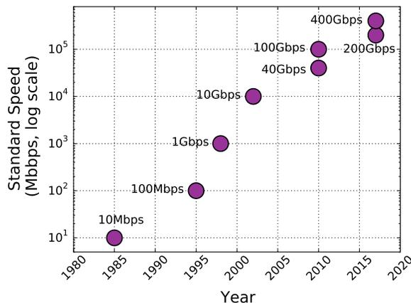
Figure 1.2: Evolution of Ethernet standard speeds. Dates refer to the year the IEEE standard for the corresponding speeds was released (not all the standards are shown).
