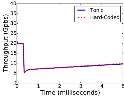
Figure 2.4: RoCEv2 with DCQCN in Tonic vs hard-coded in NS3 (40G line rate, one of two flows on a bottleneck link).
