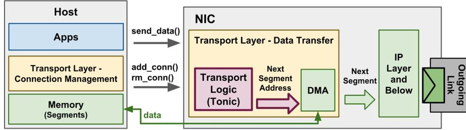
Figure 2.1: Tonic providing programmable transport logic in a hardware network stack on the NIC (sender-side).
