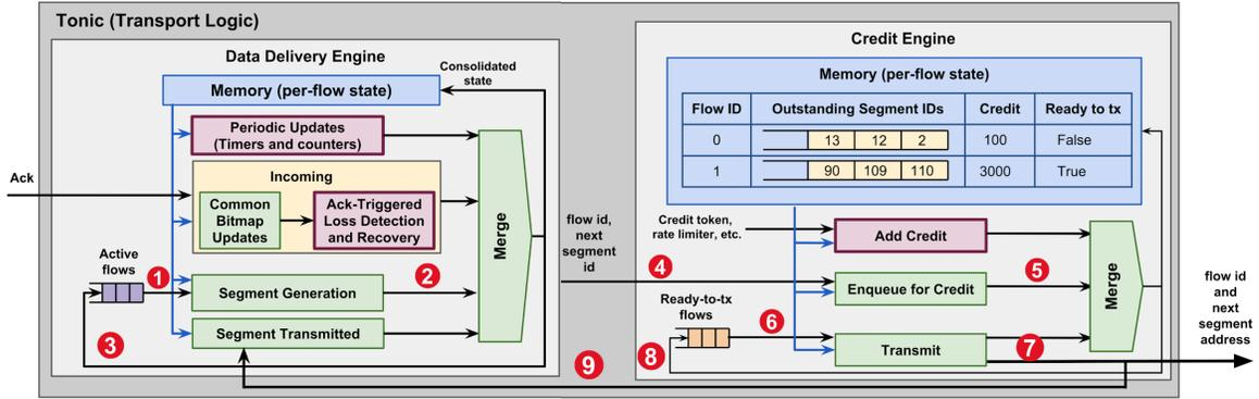
Figure 2.2: Tonic’s architecture (red boxes (also with thick borders) are programmable, others are fixed)
