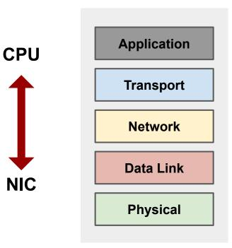
We can also optimize the movement of packets between the CPU and the NIC (FlexNIC, ASPLOS'16)
