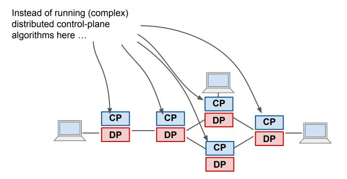
Run them here, and directly tell the switch data plane how to forward traffic.
